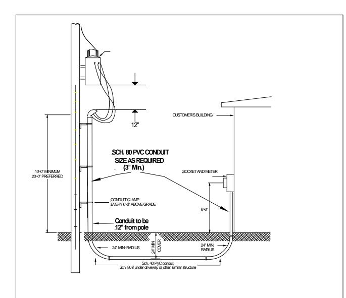
Conduit shall come straight down from meter base with one sweeping 90 below grade pointing toward source.
